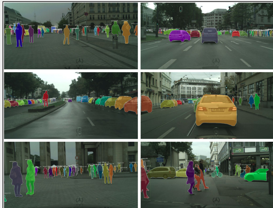
Mask RCNN applied on CityScape dataset (Reproduced with permission from Kaiming He)
